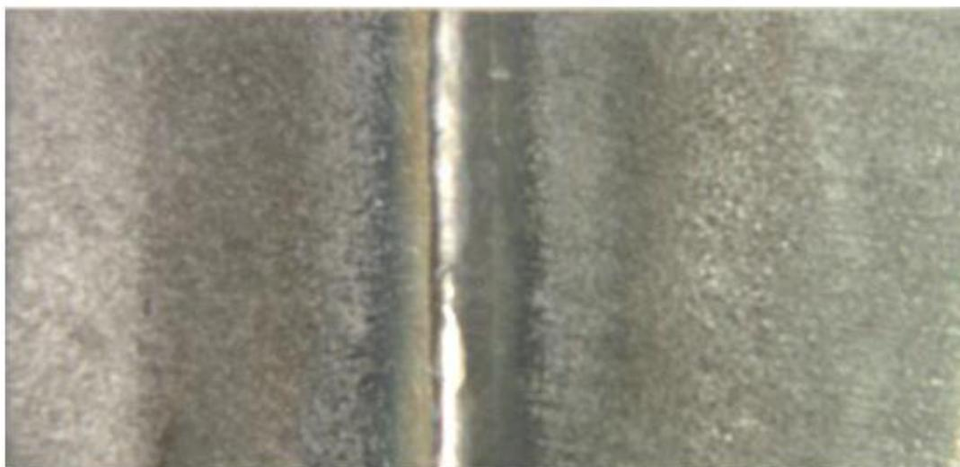
*Figure 3b: Root of weld in 25-6Mo plate welded with 625 filler metal (G48A at +50°C for 24 hours) - Pitting resistance of welds in super austenitic steels.*
