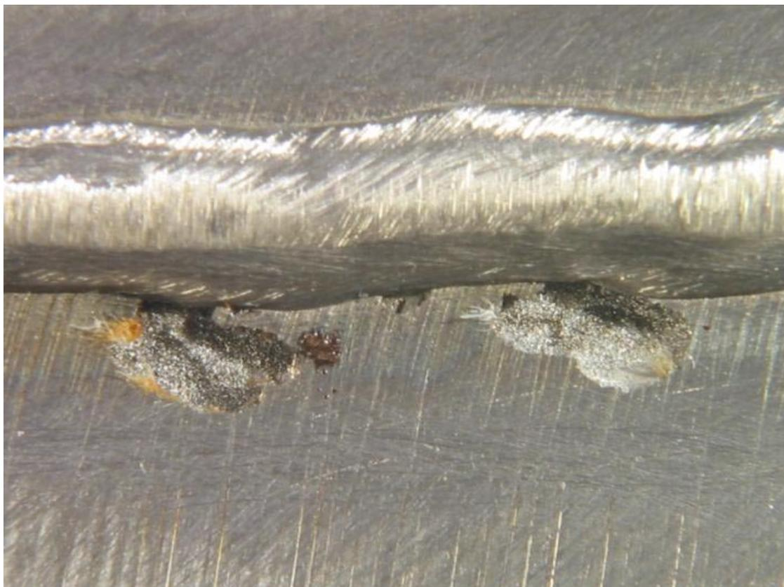
*Figure 3a: Root of weld in 27-7Mo plate showing pitting in HAZ (G48C at +70°C for 24hours) - Pitting resistance of welds in super austenitic steels.*
