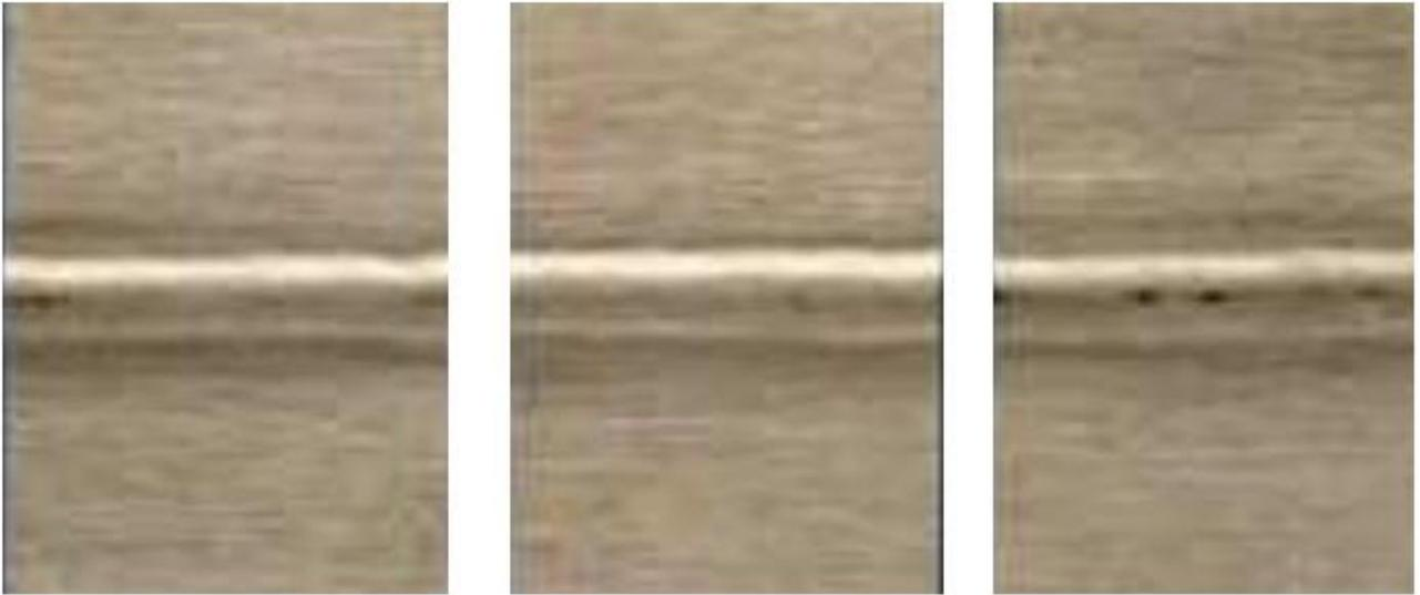
Figure 1d: INCONEL C-276 welded with INCO-WELD 686CPT filler metal (pitting resistance of various base metal and weld metal combinations).
