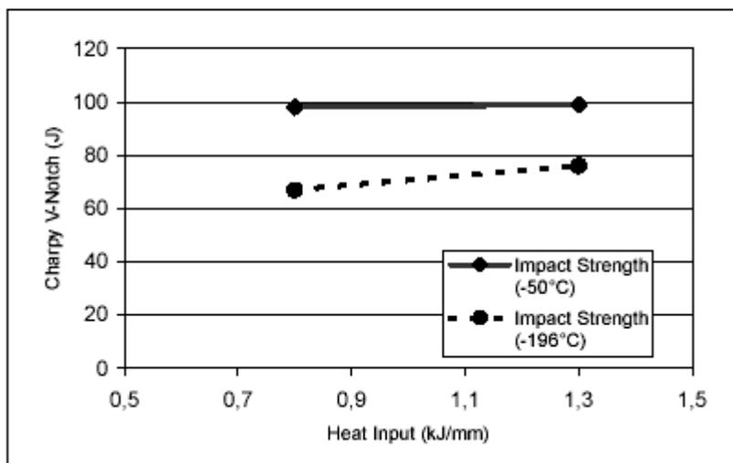
Figure 5: Variation in weld impact toughness properties for INCO-WELD 686CPT.
