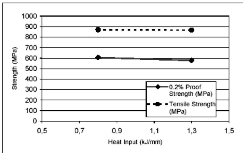
Figure 4: Variation in weld metal tensile properties for INCO-WELD 686CPT.
