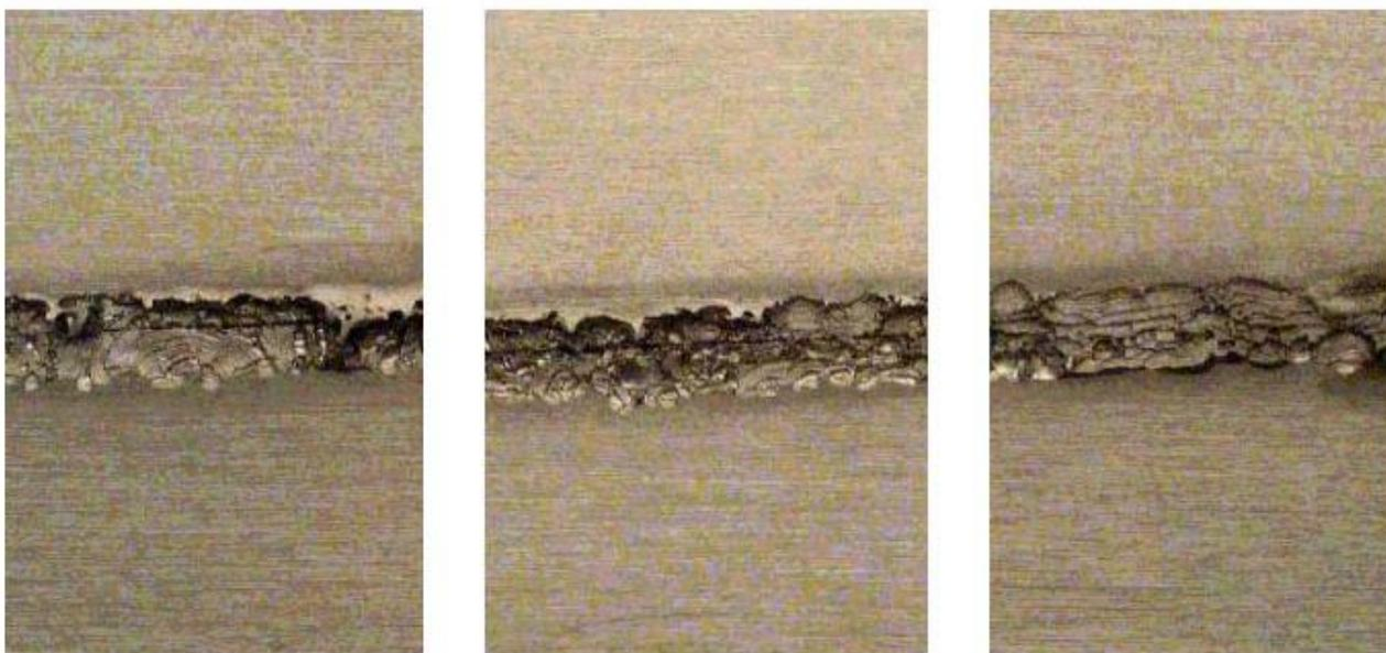
Figure 1c: INCONEL C-276 welded with INCO-WELD C-276 filler metal (pitting resistance of various base metal and weld metal combinations).
