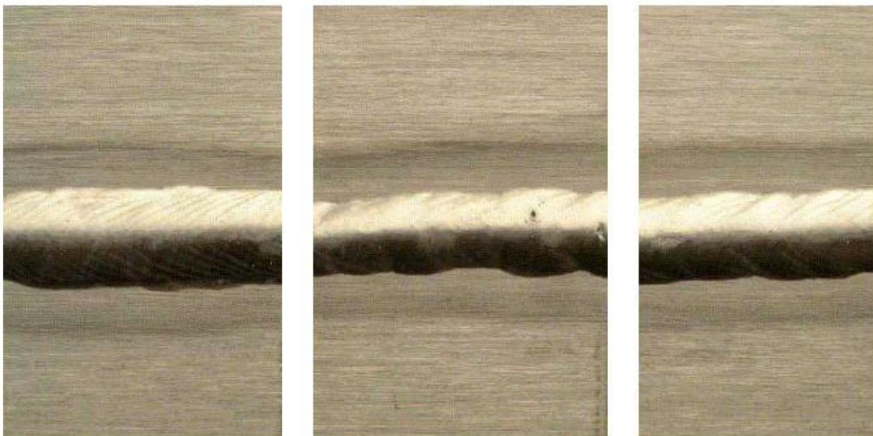
Figure 1b: INCONEL 622 welded with INCO-WELD 686CPT filler metal (pitting resistance of various base metal and weld metal combinations).
