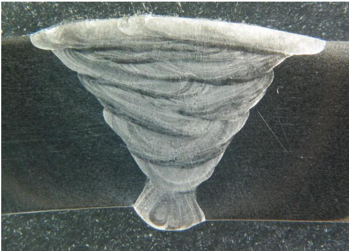
Figure 2: Macro section from a TIG weld in super austenitic stainless steel.
